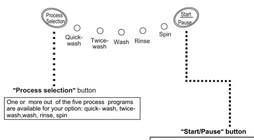
After the power is switched on, push it to start the machine
